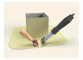
Step 10: Drop down the TPO boot over the roof curb.
